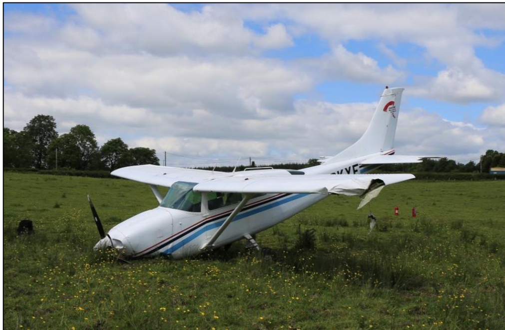
Photo No. 1: Final resting position of G-SKYE, with nose 'dug-in' and damage to left hand wing.
