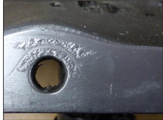
Photo No. 8: Fretting on the crankcase parting surface.
