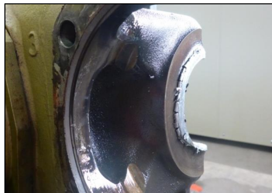
Photo No. 6: Damage to the forward face of the number three bearing housing on the 1, 3, 5 crankcase half (viewed from the cylinder side).
