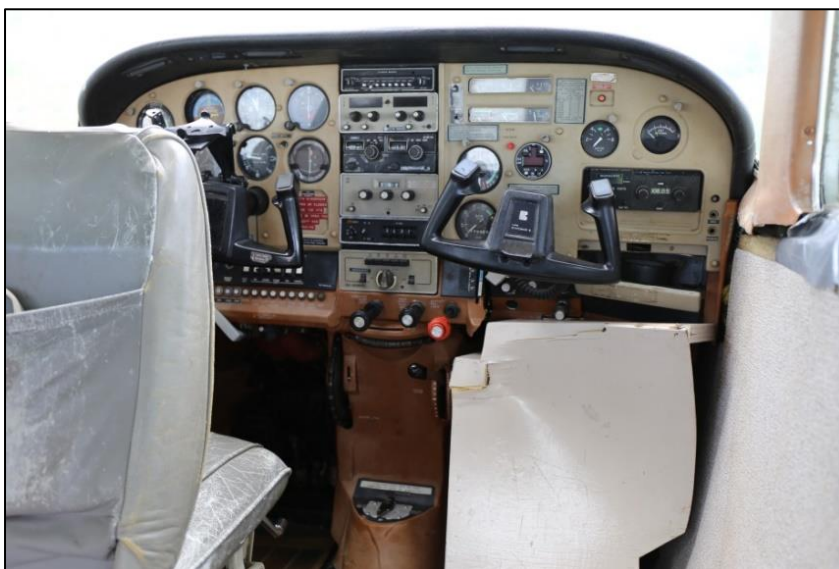
Photo No. 2: Cockpit of G-SKYE showing wooden structure at right hand foot well area.
